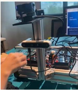
Figure 2(a) wiring the Lidar for AMR localization & Figure 2(b) setting up the stereo cameras for depth sensing
