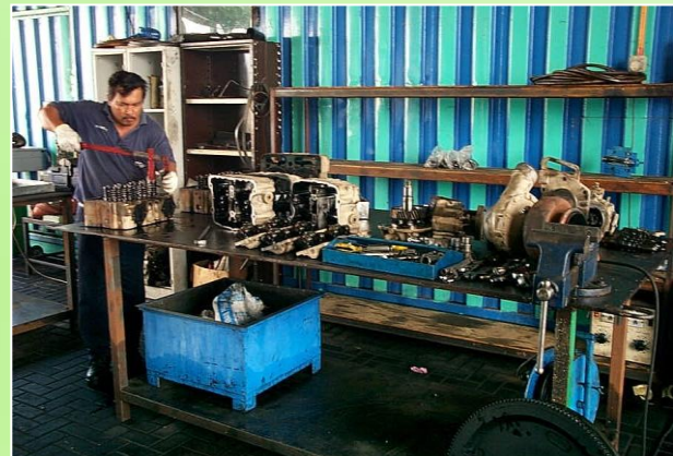
Diesel Engine Overhaul at a Port's Engineering Maintenance Workshop
