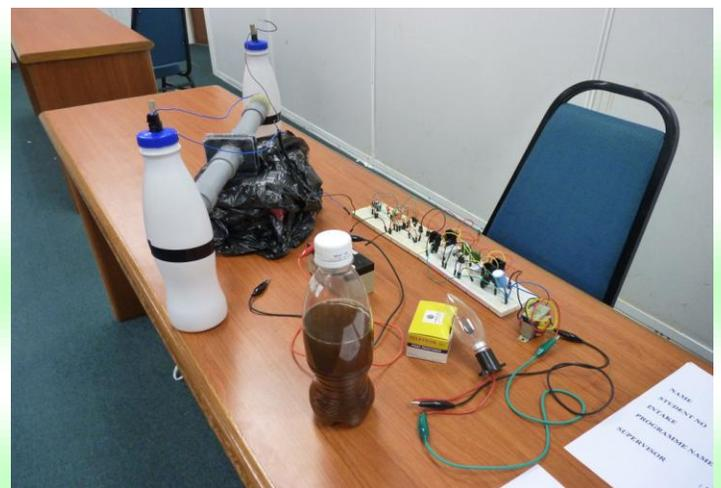
**Electricity Generation from Waste Water using Microbial Fuel Cells for Various Electrical Applications**
