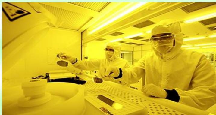
Figure 1 Dr Lai Nai Shyan performing resist coating in a class ten semi-conductor nano-fabrication clean room [4]
