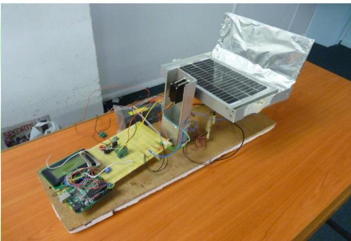
**Enhanced Ray Concentrator for Dynamic Photovoltaic Power Generation**
